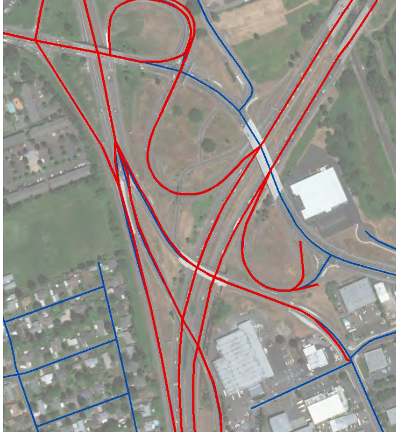
Figure 6. Highway ramps were updated, such as at this interchange between I-205 and 82nd Avenue. The 2005 ETRs (in red) are overlain on the RLIS Streets network (in blue). Inconsistencies were corrected.
